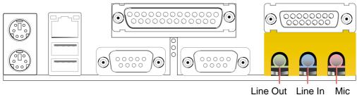
Line Out Line In Mic 1/8" Stereo Audio Connectors
